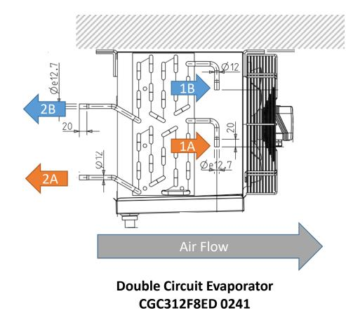
• The CO2 piping must be connected as per the above drawing ( in opposite way of air Flow)
