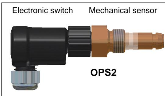
The OPS2 monitors the oil pressure differential protecting the compressor against damage if the oil differential becomes too low. Internal channels drilled through the housing link the switch to the inlet and outlet ports of the oil pump.
