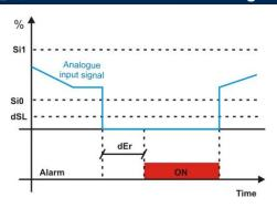
Alarm reset is automatic and happens as soon as control exceeds value set in parameter dSL. If oA1=CPr, the regulation always re-starts after expiring both anti-short cycle timers 2on (minimum time between two consecutive compressor activations) and 2oF (minimum time between one compressor stop and next start-up).
