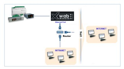
Before connecting XWEB-EVO to the network, make sure that the IP address you wish to use for XWEB-EVO has not already been claimed and can therefore be used. You can run a PING on that address, and if you receive at least one reply the address needs to be changed, as this means it is already in use.
