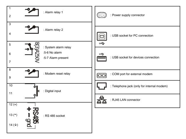
**NOTE**: for XWEB500, the 'reset modem' relay is energised for a reset every two minutes in the event of inactivity, and before each use (sending of a fax, dial-up, etc.). Add this relay to the power supply circuit of the external modem to guarantee the correct transmission of messages (e.g. SMS messages).
