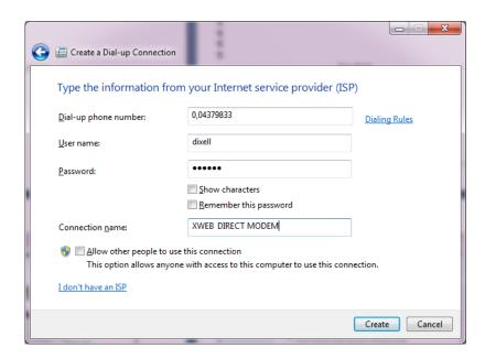
Enter the telephone number of the line that XWEB-EVO is connected to. If there is a switchboard and the number that needs to be dialled for the external line is 0, enter: 0,04379833. Enter 'dixell' as the user name and password connection parameters. Enter a name to identify the XWEB-EVO that you wish to contact with the call.
